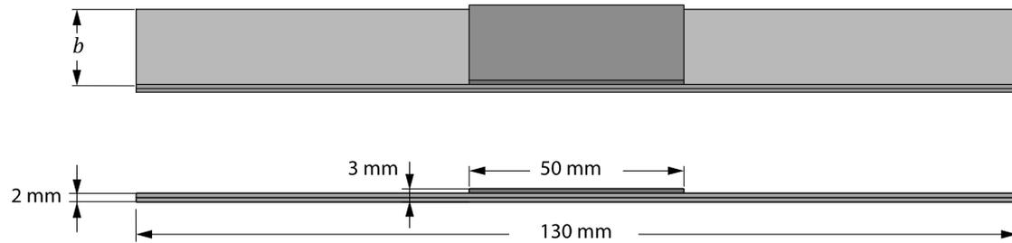
Figure 1: Illustration of the ply-drop specimen including nominal dimensions
